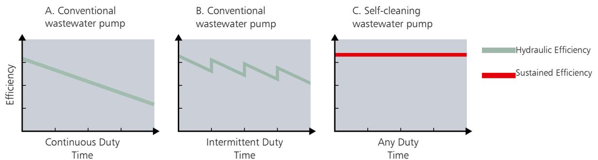
Non-clog pump performance under two different operating scenarios compared with a self-cleaning wastewater pump
