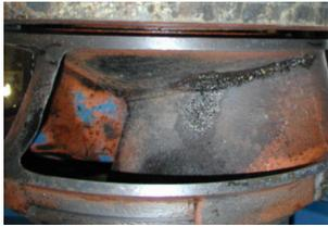
Figure 13: On this impeller, cavitation damage is located near the hub on the pressure side of the blade. In this case the pump has been operated in the recirculation region; matters have been worsened with speed variation and a flat system curve.
