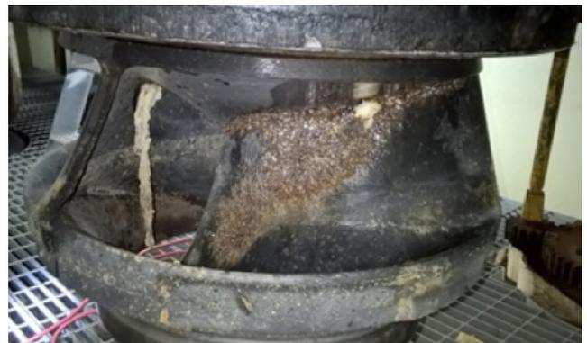
Figure 1: Cavitation damage on the blade of a centrifugal pump impeller.
