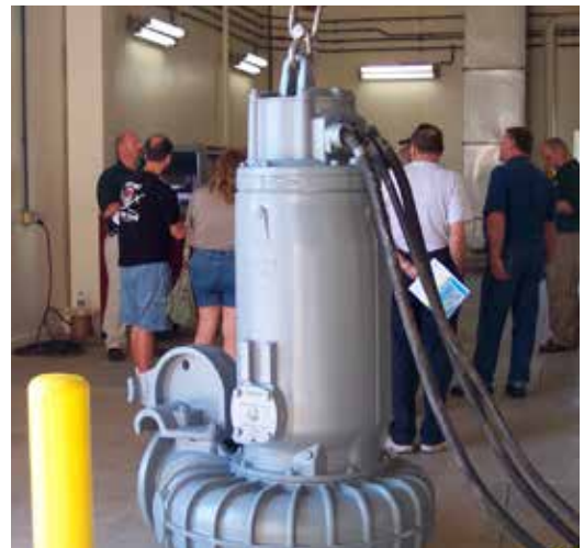
Flygt provided 26 pumps for the project, including the influent pump shown here.
