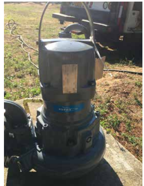
Concertor trial pump ready to be installed
