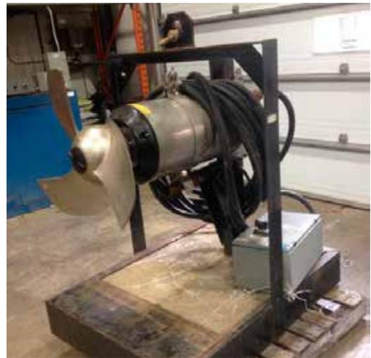
A Flygt 4680 submersible mixer was installed to discourage ice from forming near the cables.
