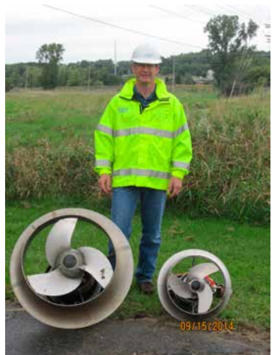
Compact low-energy Flygt mixers (right) replaced larger mixers (left).
