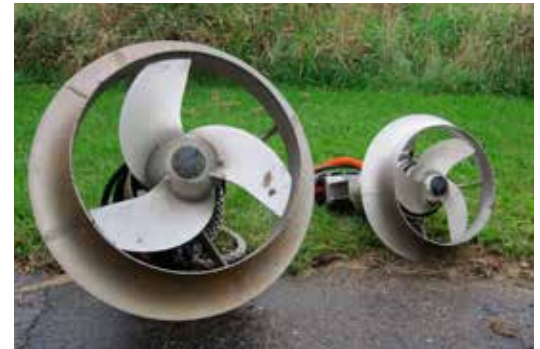
Xylem proposed replacing the large mixers (left, Flygt Model 4650, 7.5 HP) in the biological selector basins with smaller, lower energy mixers (right, Flygt Model 4630, 2.5 HP).
