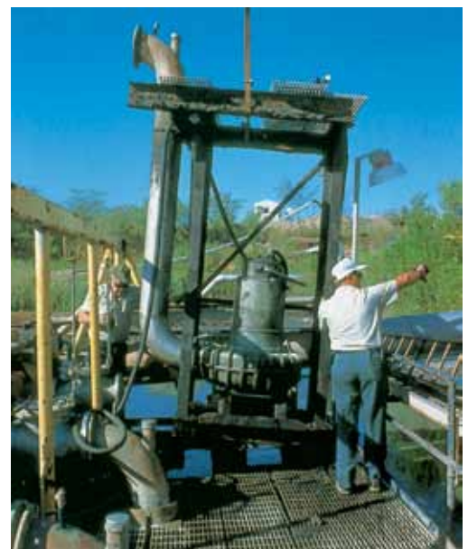
By simply removing the bolts securing the discharge pipe to the manifold, the entire pump-discharge module can be hoisted up, for fast and easy access to the pump
