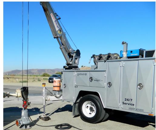
Xylem service truck with a crane, making installation and pump positioning easier for the Xylem team.
