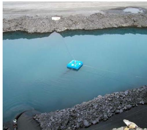
Flygt pump rafts enable adjustment to water level fluctuations. The larger image shows the pump and floatation raft working together in a mine drainage application.
