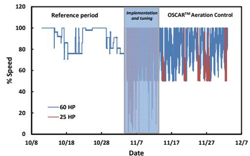
Figure 2: Aerobic basin DO concentration over time. 100% speed corresponds to 1500 scfm for 60 HP blower and 700 scfm for 25 HP blower.
