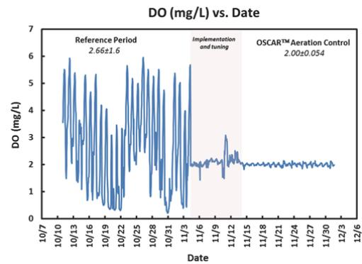
Figure 1: Aerobic basin DO concentration over time.
