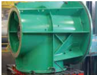
Restoring the registered fit and mounting flange flatness, and parallelism of a discharge elbow from a 102 x 72 WCA pump.
