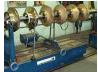
Balancing the rotating element for an 18 x 10 CDV 6 stage pump.
