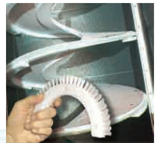
Durable segmented brushes make replacement easy.
