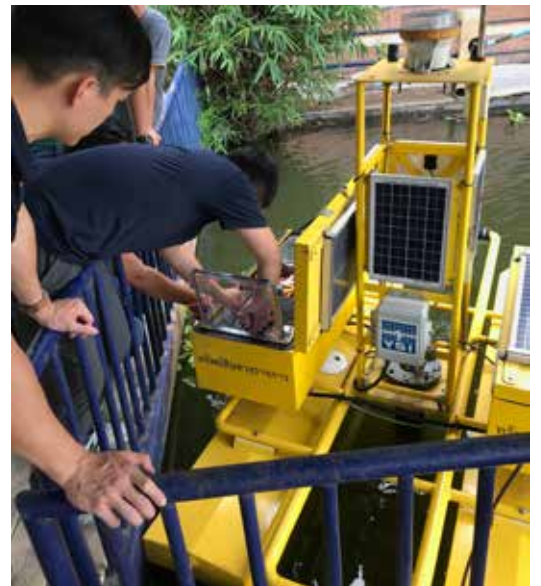
Figure 5: Xylem YSI and Green Banyan personnel providing monthly servicing of PISCES buoy
