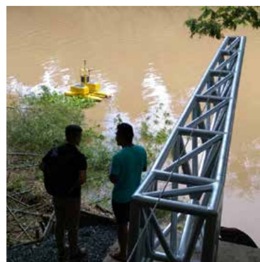
Figure 7: Custom support frame for high flow events
