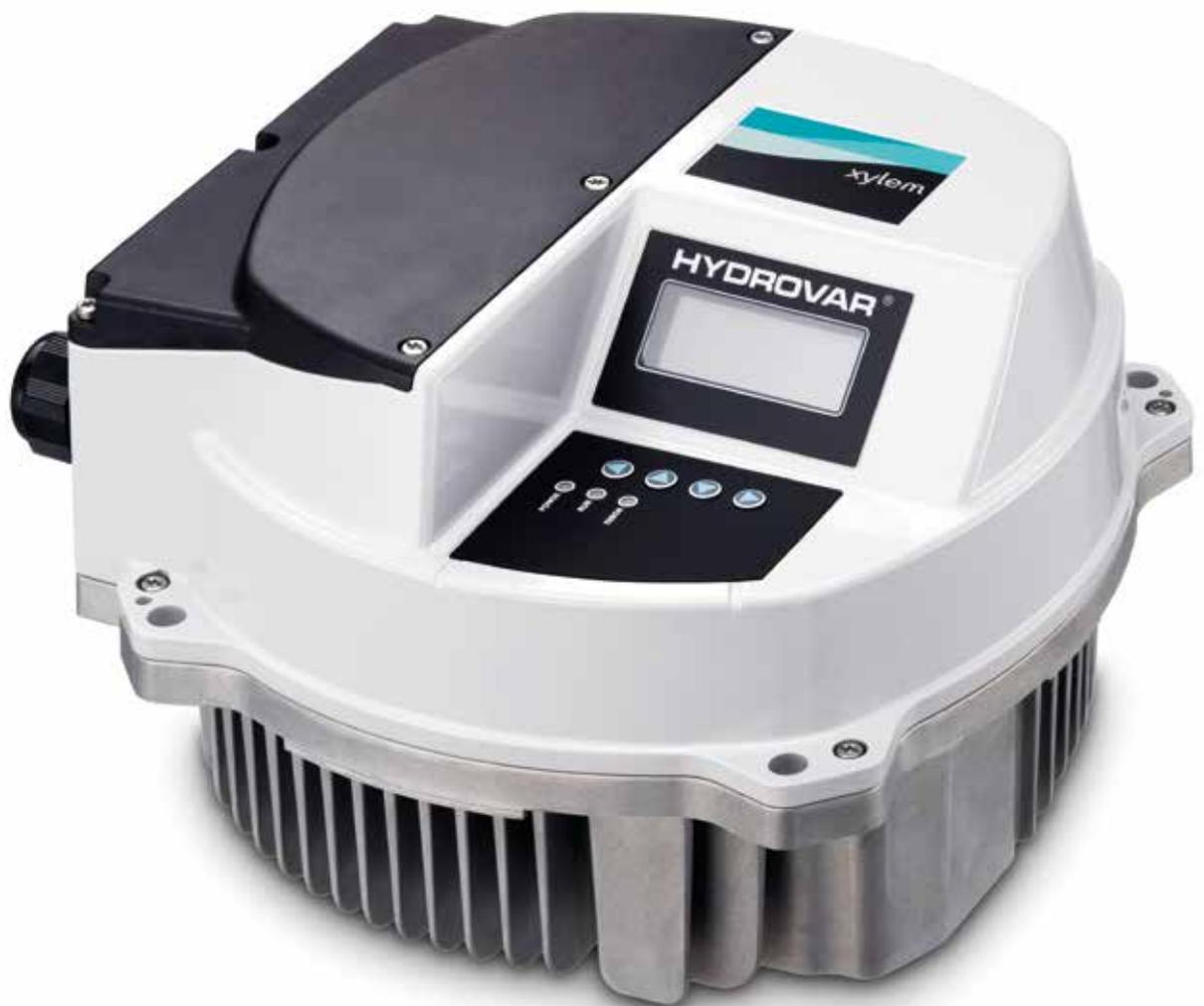
Retrofitting the 'plug and play' HYDROVAR units to a fixed speed booster set not only eliminates the need for a control panel but also introduces a soft start function, that when combined with the benefits of running a pump at a variable speed, can prolong the life of the pump and the water system. By reducing the in-rush current when the pump is turned on, parts such as motor bearings and pipe fittings are protected from hydraulic shock that can cause cavitation and breakdown.
