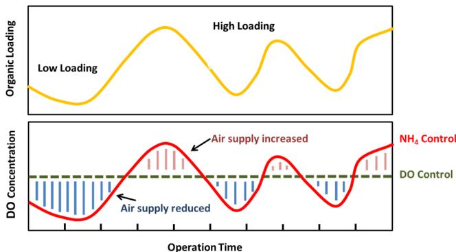
Figure 3. Air supplied with DO and Ammonia sensor control systems.
