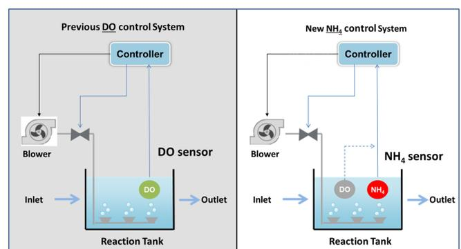
Figure 2. Comparing DO sensor aeration and Ammonia sensor control systems.
