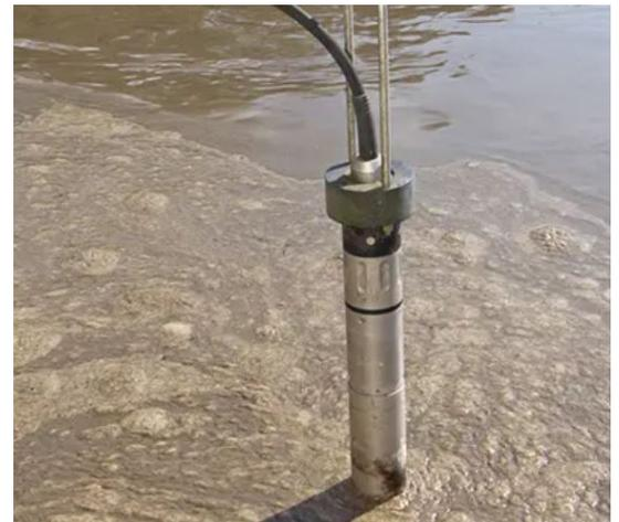
*Ammonium ISE sensors are popular in wastewater for the enormous benefits they can bring to the treatment process at an affordable price. With continuous ammonium measurements, automatic control of aeration can be immediate and proportional to the incoming ammonium load.*
