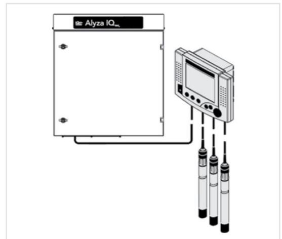
*WTW Alyza IQ Analyzers connected to the MIQ/TC 2020 3G (terminal controller) with MIQ/JB (module for system expansion).*
