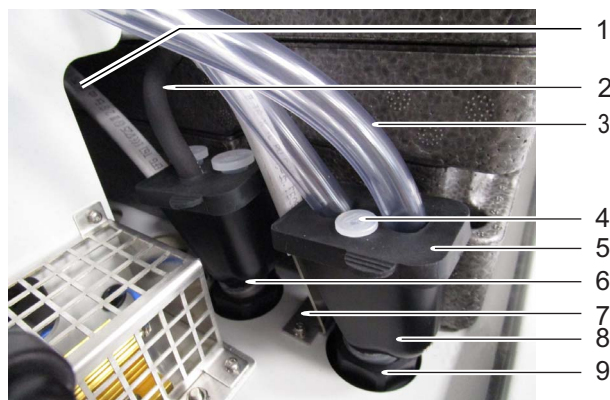
figure 3-26 Collection funnel for the separate discharge of all liquids
