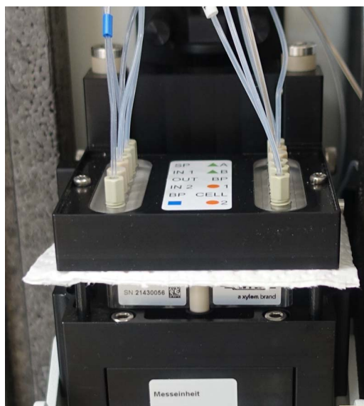
figure 5-5 Removing the liquids remains with absorbent, lint free paper
