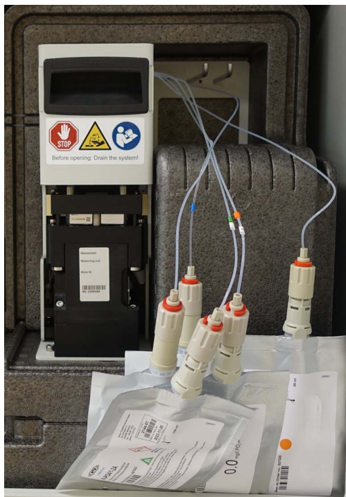
figure 5-6 ChemBags removed to be exchanged
