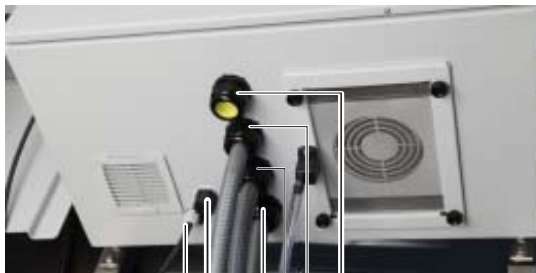
figure 3-24 Connections at the housing bottom (from below) Example: 1 sample channel, 1 drain, 1 trigger cable
