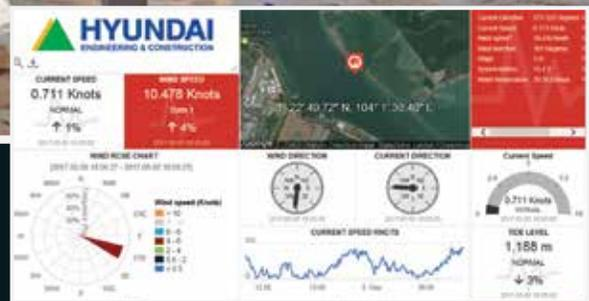
The real-time data dashboard used to alert operators of rapidly changing, potentially dangerous conditions.
