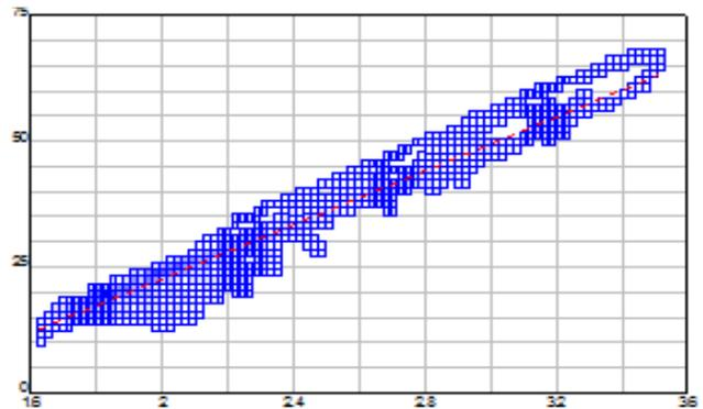
Downstream site with tidal affects during low flows and multiple loop stage to discharge rating
