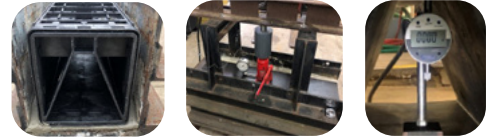
Type S recycled underdrain passes the downward loading test
