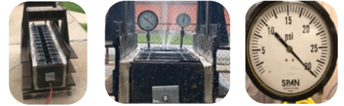
Type S recycled underdrain passes the grouted internal burst strength test
