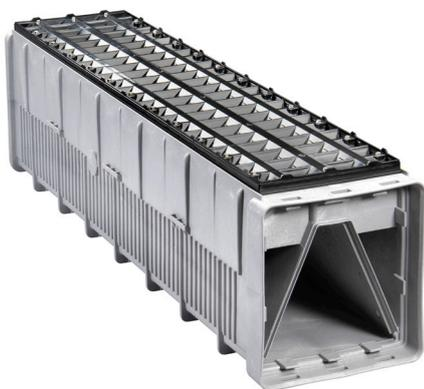
The Leopold Type S underdrain with I.M.S.® 1000 media retainer provides superior air and water distribution and retention of monomedia sand particles greater than 1.7 mm.
