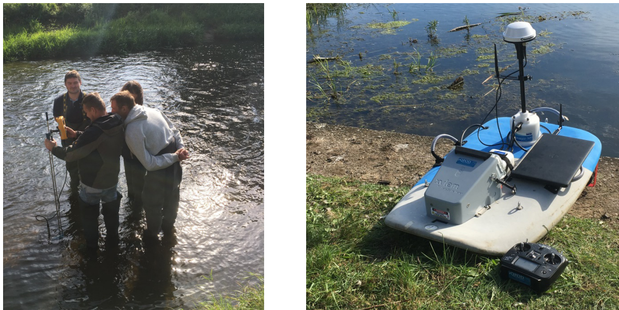
FIGURE 2. Falk with some clients and a Flowtracker 2 (left), rQPOD with M9 ADCP (right)
