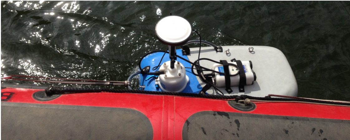
FIGURE 2. The HydroSurveyor Mounted on the Torrent Board and Towed Alongside.
