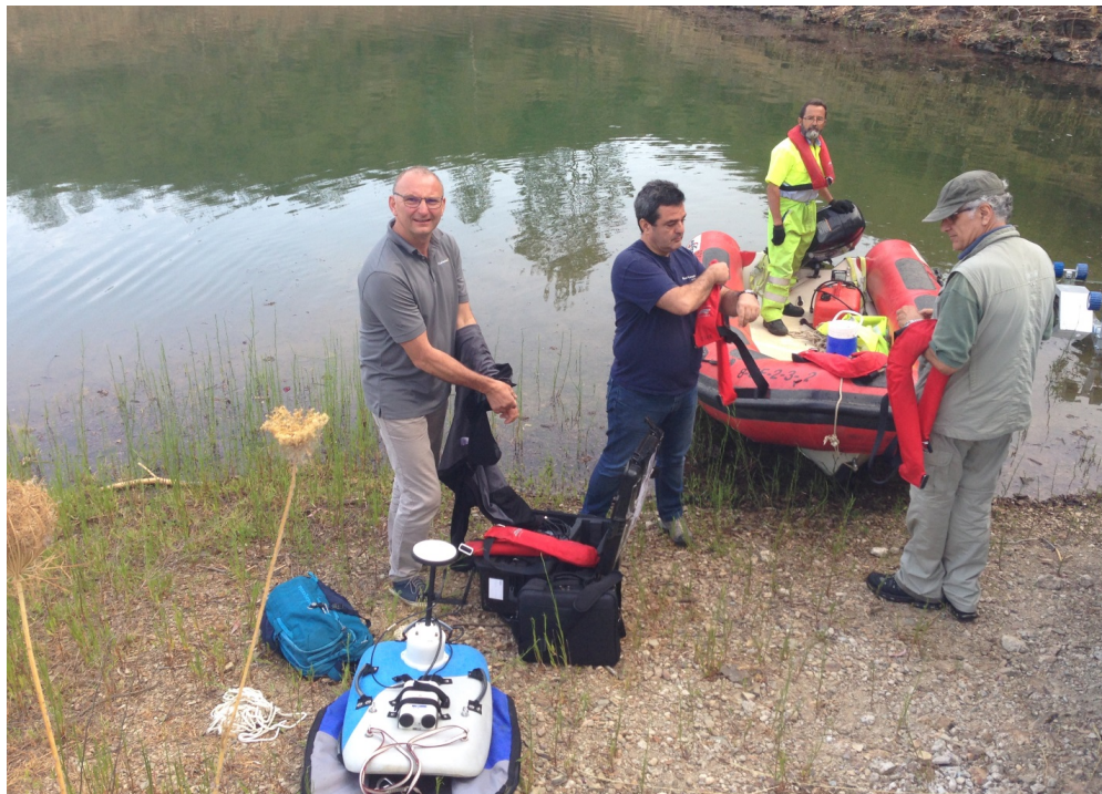
FIGURE 1. Setting up the survey boat! The HydroSurveyor installed on a Torrent board is shown in the front.
