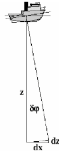
FIGURE 13. Pitch angle artifacts in the Profile window in Phase 3 of editing in the HYSWEEP® Editor.
