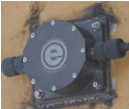
Inclinometer Mounted on Boom
