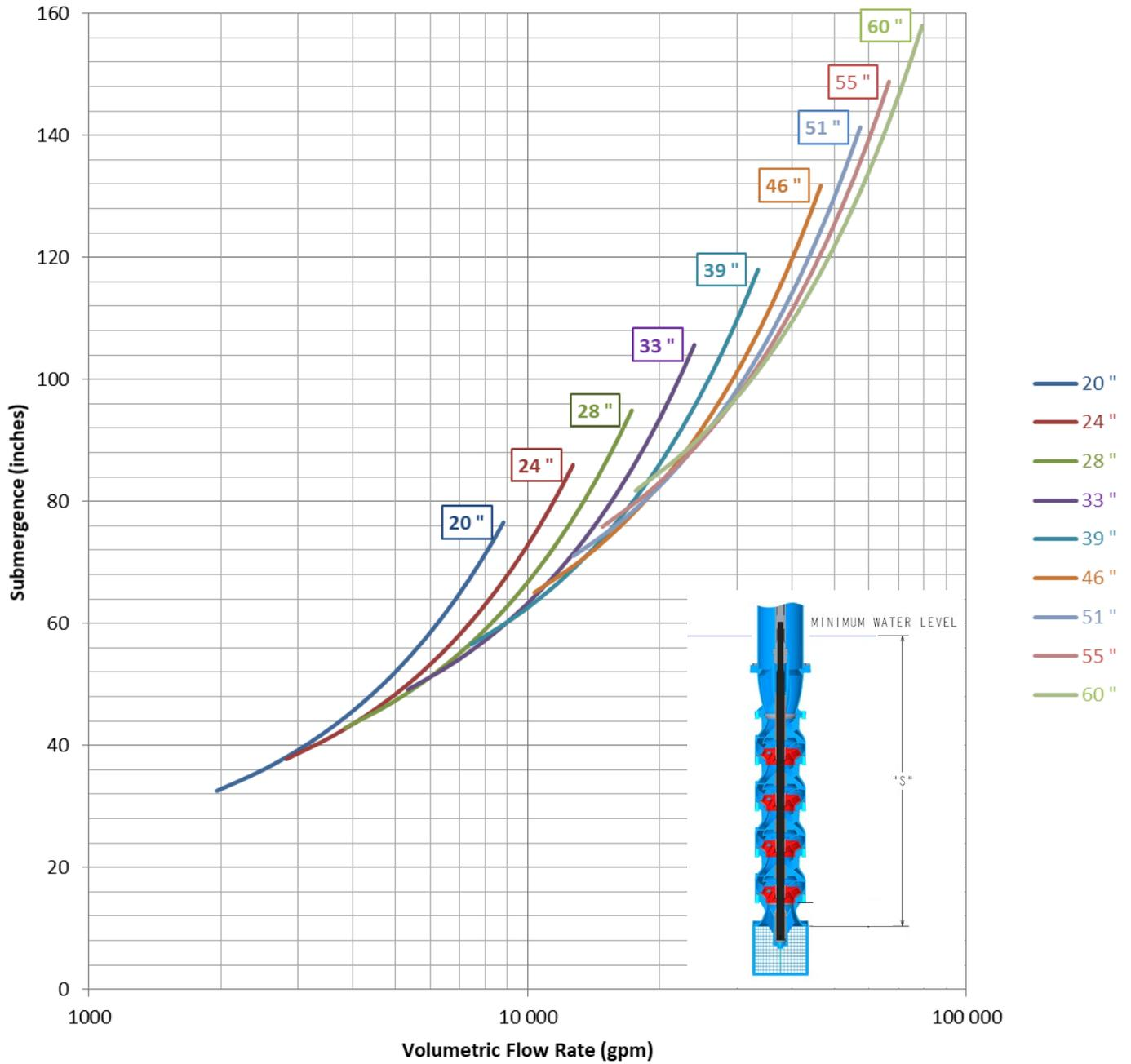
Figure 2 - Minimum Submergence Curves - Diameters 20" - 60" – Imperial Units
