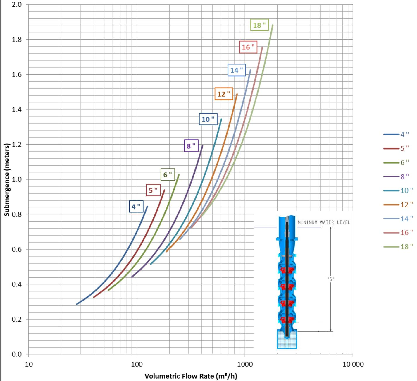
Figure 3 - Minimum Submergence Curves - Diameters 4" - 18" - SI Units
