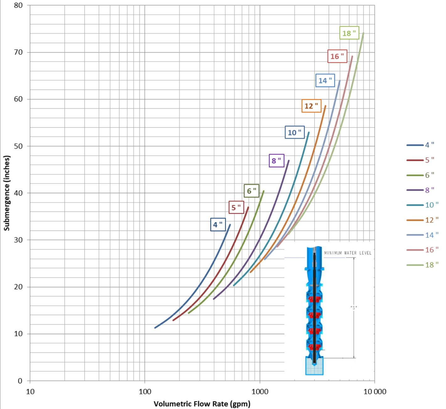
Figure 1 - Minimum Submergence Curves - Diameters 4" - 18" – Imperial Units
