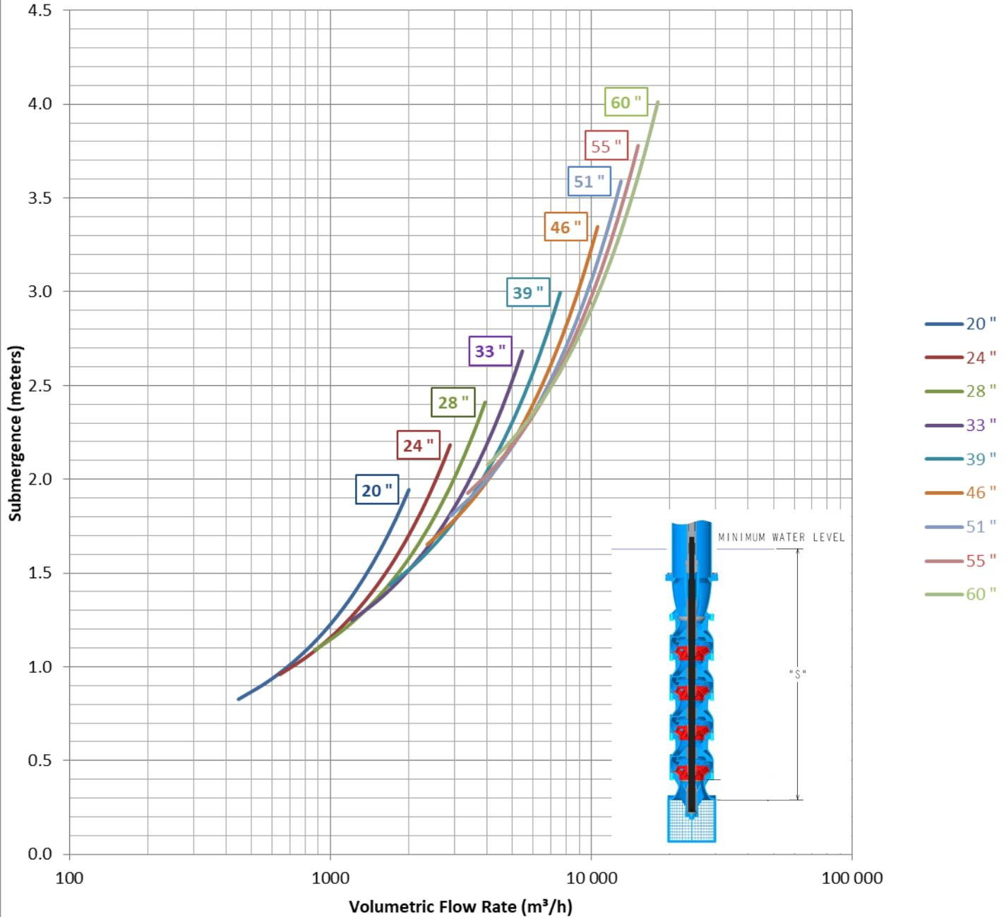
Figure 4 - Minimum Submergence - Diameters 20" - 60" - SI Units
