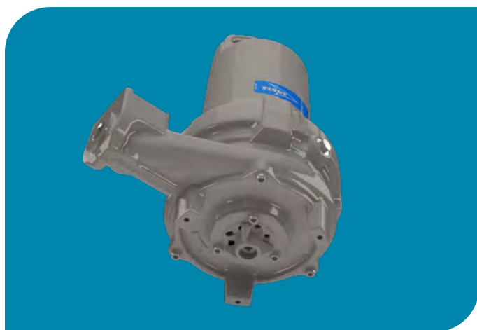
Figure 8.1.3: Centrifugal grinder M3090, typically 1 l/s @ 43 m and 13 Amp (16 USPGM @ 140 feet, 22 Amp).
