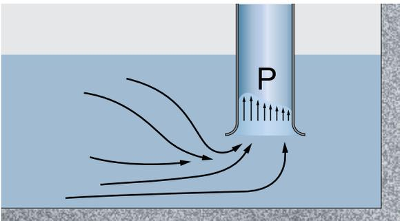
Uneven velocity into the pump inlet.
