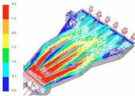
CFD simulation of modified design.
