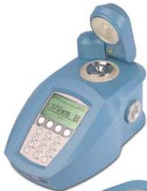
Digital Refractometers with Peltier Temperature Control for chemical, pharmaceutical and petrochemical applications.
