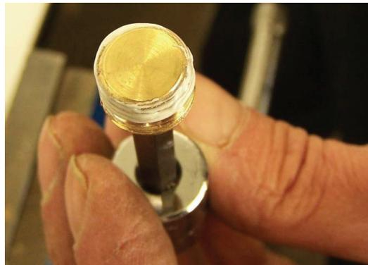
4. If Loctite 567 is unavailable, we recommend Rector Seal No. 5 pipe thread sealant for all non-glycol based applications, or any PTFE thread sealing tape. Be sure to follow the manufacturer specific handling precautions and application instructions as noted on the product labeling.
