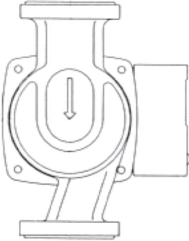
The water has to squeeze through this smaller opening to get out of the volute. The effect you get is similar to what happens when you put your thumb over the end of a garden hose. The velocity increases, doesn't it? Well, that velocity is the force that moves the water around the system. It's the force that overcomes the system's pressure drop.
