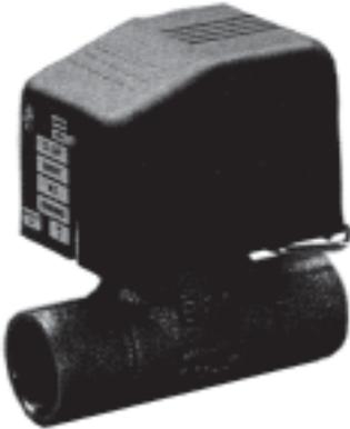
Another way to zone a hot water system is to use electric zone valves with a single circulator. The zone valve takes the place of the Flo-Control valve. Each zone valve acts as a “Gatekeeper” to the zone it serves. The circulator provides the water, and the zone valve allows that water to either pass or not pass.
