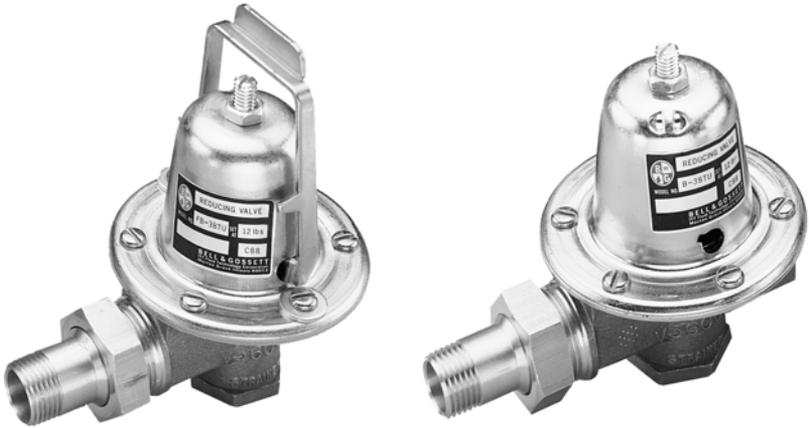
The pressure-reducing or “feed” valve’s job is to fill the system with water and to keep that water under a few pounds of pressure at the top floor. Your job is to figure out how much pressure you need in the basement to push the water up to the top of the system and hold it there under pressure.
