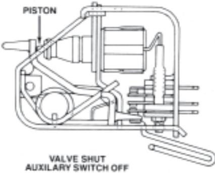
That switch cuts power to the heat motor, and almost immediately, the wax in the power pill begins to cool and shrink. Naturally, as that happens, the spring-loaded lever arm pushes the piston back into the power pill. The circulator, however, is still
