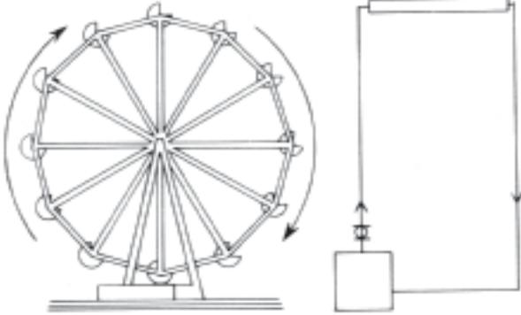
When a Ferris wheel turns, the weight going up balances the weight coming down. There's no lifting going on here, there's only turning. That's because everything is in perfect balance. The Ferris wheel's motor doesn't have to do any lifting. All it has to do is overcome the friction in the bearings (and in the air, of course) to set the big wheel in motion.
