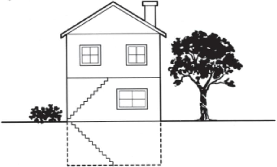
You've installed the feed valve in the basement, naturally. You've piped it at a convenient height, say, about four feet below the basement ceiling. Now, let's figure out how high the feed valve has to lift water to get it to the top of the system in this house.
