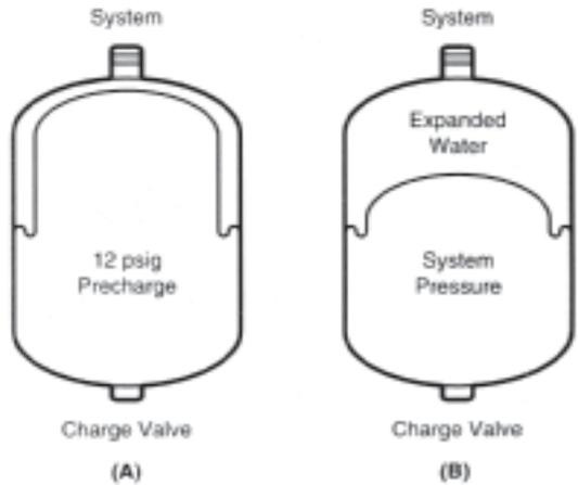
and squeezes it like a balloon. As long as the tank is in good working order, the water and air never touch each other. Should the diaphragm fail, however, the tank will lose its air cushion and the relief valve will almost surely pop on the next firing cycle.
