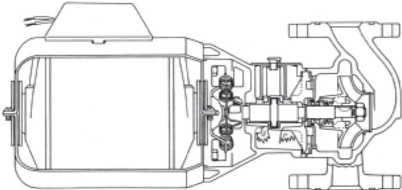
The Series 100 circulator has a bearing assembly that holds the pump shaft. The shaft spins at 1,750 rpm on two, quiet-operating sleeve bearings. You should always use SAE-20 non-detergent oil on sleeve bearings. Don't use detergent oil because detergent builds up over time, and since it has no lubricating properties, it can lead to bearing failure.
