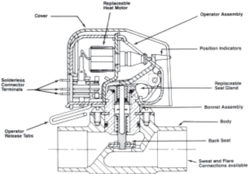
First, the room thermostat calls for heat by sending an electrical “Go” signal to the zone valve’s operator. Inside the operator, the electricity flows through a normally closed switch and around a tightly wound coil called a heat motor. This wire has high resistance, so when the current flows through it, you get heat.
