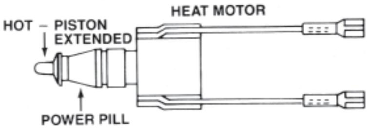
The piston pushes against the spring-loaded lever that normally holds the valve closed. This action lifts the valve disc off its seat and opens Comfort-Trol’s water valve. Water now has access to the zone. But nothing is flowing because the circulator hasn’t yet been called on by Comfort-Trol’s operator. That’s about to happen, though, because the piston will keep pushing the lever forward until it trips an end switch.
