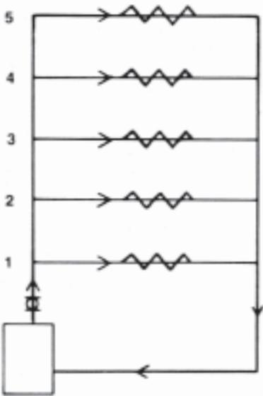
Today, most of your systems don't have open tanks in the attic; they have "closed" steel compression tanks or diaphragm-type tanks, and most of the time, these tanks are down in the basement. You don't pour water into the system from the top any more, do you? No, you force it up from the bottom. And that's where the pressure reducing valve comes in.
