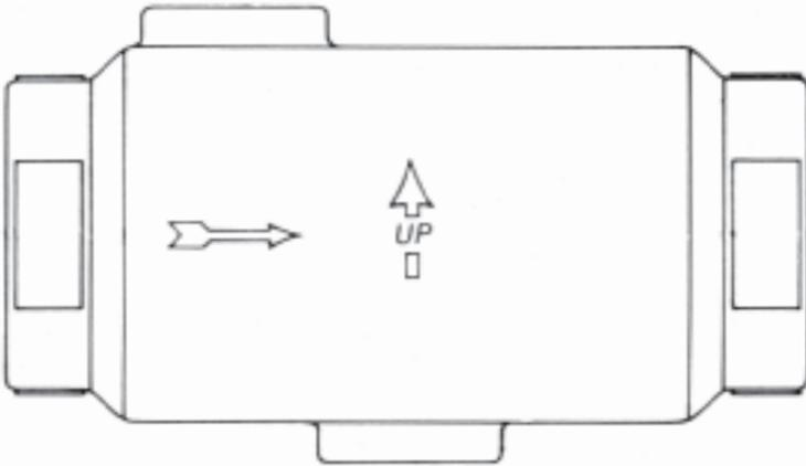
that’s a bit smaller than the chamber itself. Air-laden water flows through the pipe and enters the “wide space in the road” — the IAS. Naturally, as the water widens out in the IAS, it also slows down. That slowing motion releases the air bubbles in the same way a slowing river current releases floating debris.
