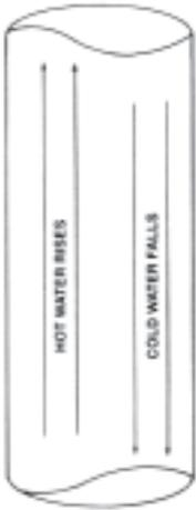
The hot and cold water just flow past each other in the same pipe. You'll usually notice this "back end" gravity circulation if there's a radiator directly above the boiler on the return side. Adding a second Flo-Control valve to the return side of the zone piping will solve the problem every time.
