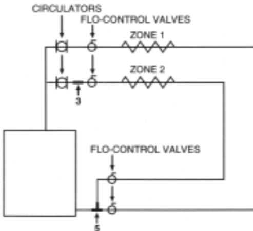
Can you see it? Some of the return water from Zone #1 is moving backwards through Zone #2. How do you solve the problem? Just unscrew the top of the Flo-Control valve and clean it out. Easy!
