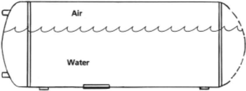
sizing, the pressure will usually rise only a pound or so by the time the system reaches its high-limit temperature.
