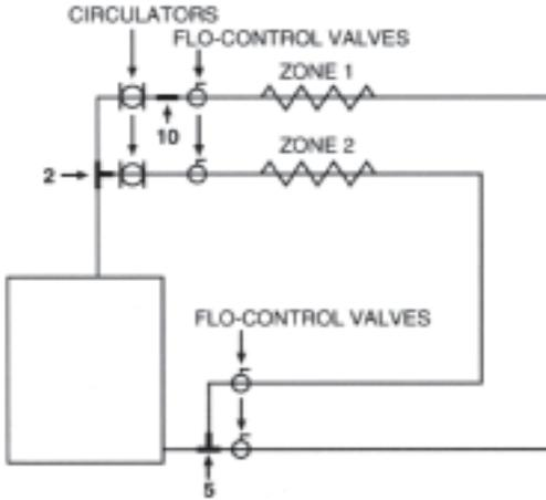
Let's say the strength of the circulator at its discharge flange is "10." As water flows, friction eats up some of the circulator's power. By the time it reaches the return tee, the circulator's strength is down to "5." Now the water flows through the boiler and out the supply header. Its strength at the supply tee leading to the two zones is down to "2."
