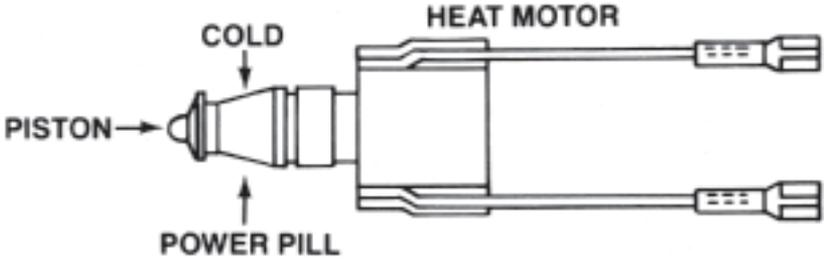
The power pill is filled with a temperature sensitive wax that expands when the heat from the heat motor hits it. As the wax expands, it pushes a piston out of the power pill.
