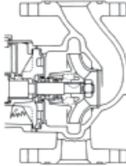
The circulator, like the rest of the closed heating system, is always filled with water. There's no way it can ever empty itself of water when it's running. All it can hope to do is toss out what's currently inside of itself.
