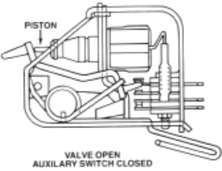
The end switch makes a connection (through a relay) back to the circulator. The circulator instantly comes on and moves water through the Comfort-Trol water valve and out to the zone. In systems without
