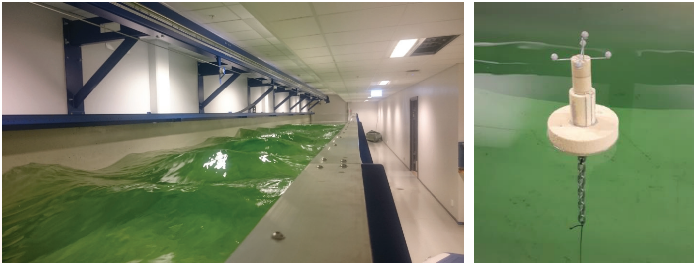
Figure 5: Tank test facility. Validation of the IMU in tank reference system and optical reference system
