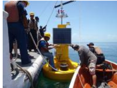
The size of the buoy allowed for easy deployment from small vessel (36x8m)
