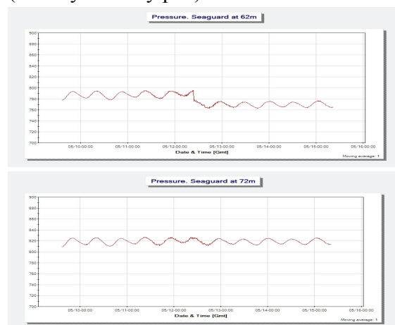
Figure 3. Pressure record from the Seaguards at 62m and 72m from May 10 th to May 15 th
