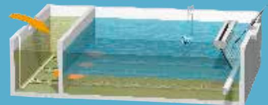
**Settle phase:** Basin agitation from the react phase (i.e. aeration and mixing) is stopped to allow the solids to settle to the bottom of the basin. Raw wastewater continues to flow into the pre-react zone while the main react zone settles. As the solids settle, a clear layer of water develops on top of the basin.
