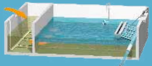
**Decant phase:** The decanter descends gradually downward to draw off the clarified supernatant. Wastewater continues to flow into the pre-react zone as the treated and clarified effluent is decanted from the main react zone at a constant rate. Waste activated sludge is typically removed from the basin during this phase.
