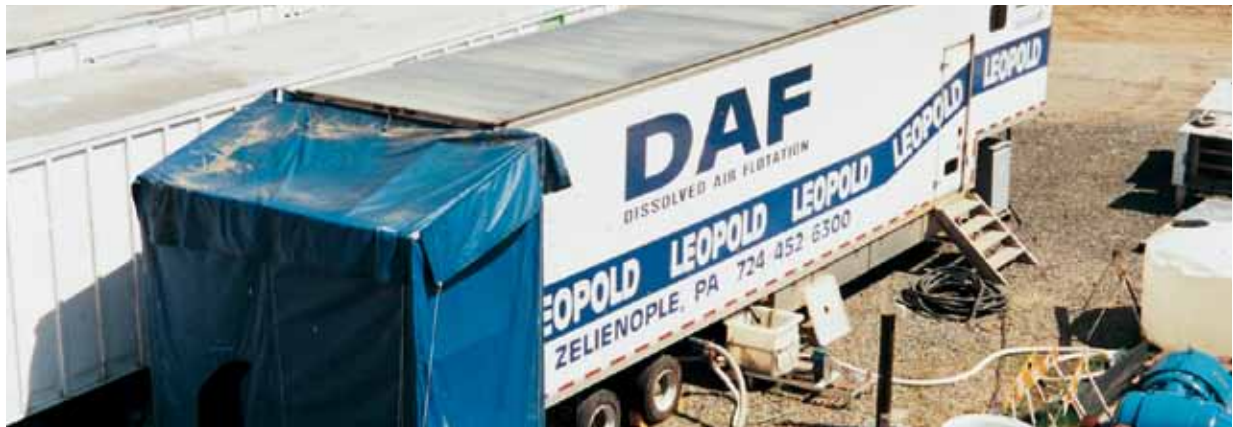
The Leopold® mobile Clari-DAF® system pilot plant gathers data every five minutes around the clock for weeks under actual operating conditions to determine the most appropriate flocculation conditions for designing and engineering a full-scale Clari-DAF® system installation.
