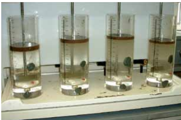
The Leopold® Jar Testing Unit is a stand-alone system designed to test four samples independently and simultaneously, giving flexibility and variable control.
