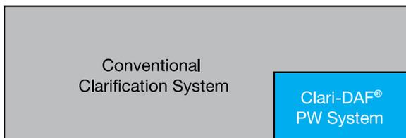
At one-sixth the footprint of a conventional clarification system, the Clari-DAF® PW system in South Carolina handles twice as much annual flow at a treatment cost that is 41% less.
