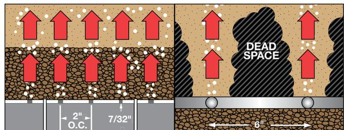
The closely spaced, non-clogging orifices designed into Leopold Type S Technology Underdrain (left) provide uniform distribution of air and/or water backwash for trouble-free operation. With orifices widely spaced, dead spaces and inefficient cleaning of the media can occur.
